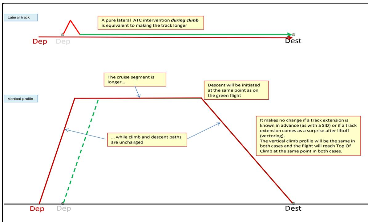
Figure 1. CCD and lateral extension of the flight in climb phase.
