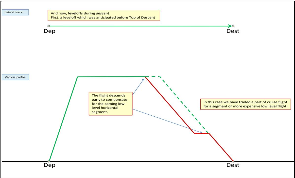
Figure 5. A leveloff segment in the descent phase, known well in advance of ToD.
