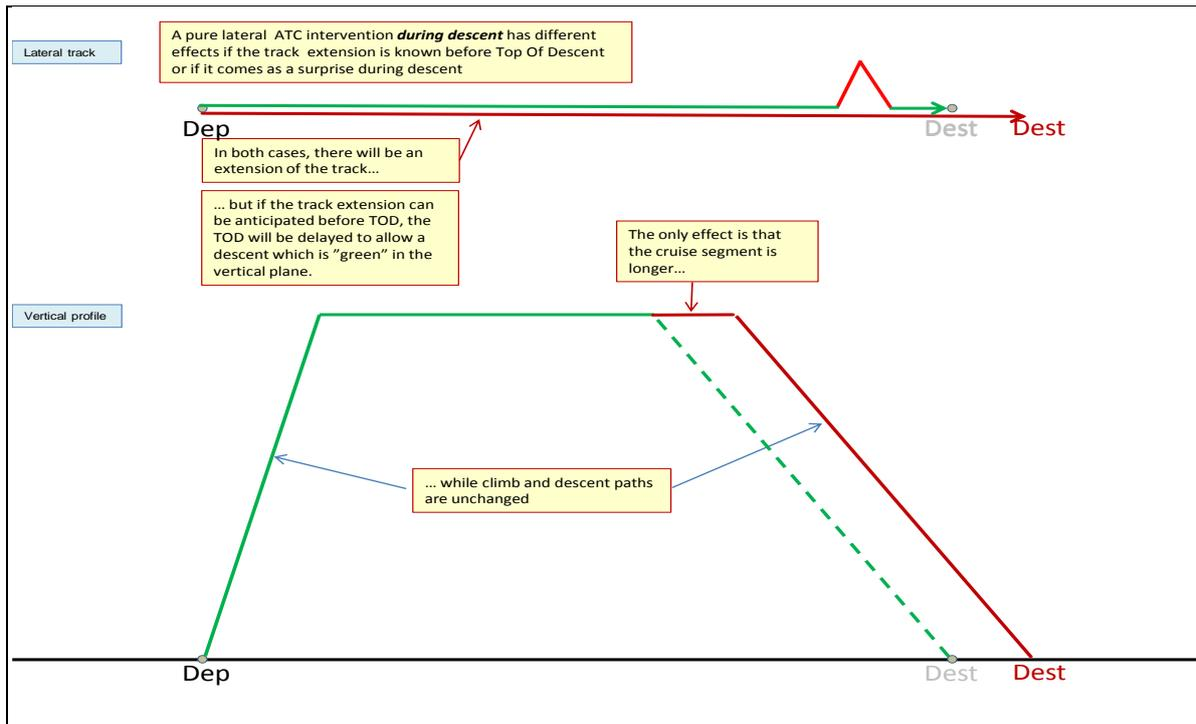
Figure 2. Influence of lateral extension on the trajectory before the ToD.
