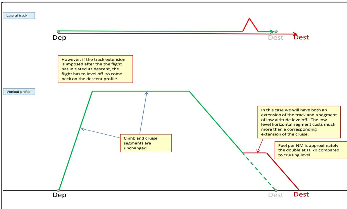
Figure 3. Influence of lateral extension on the trajectory after the ToD.
