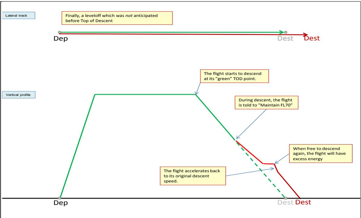
Figure 6. A leveloff introduced after the ToD, not known in advance.
