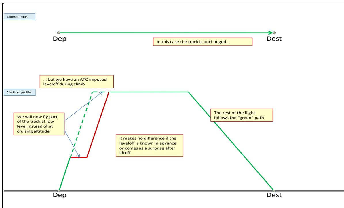
Figure 4. A leveloff segment in the departure phase of the flight mission.
